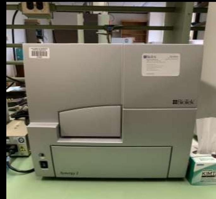
Fluorescence Microplate Reader used to quantify cellular attachment
