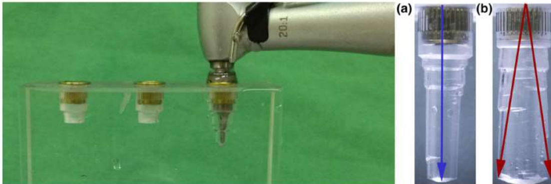
Fig. 3. Image taken by digital camera showing the resulting cavity after drilling in the centric position (a) and after applying eccentric forces (b).
